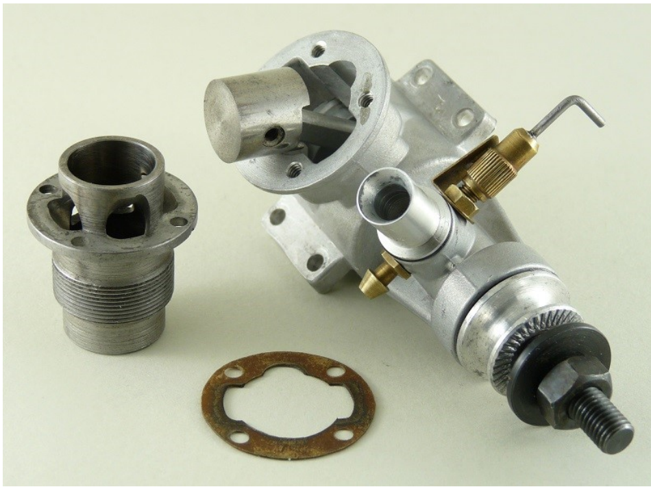
Dismantled experimental version shows Schnuerle ported cylinder and other modifications.
