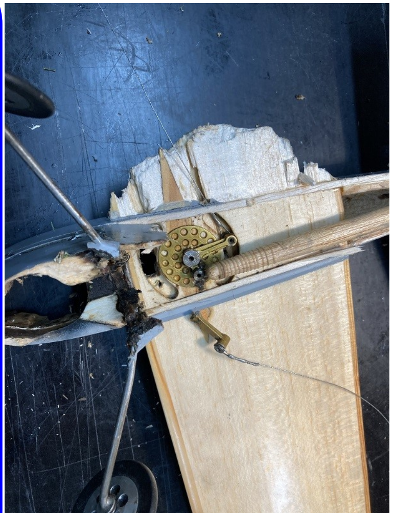
This substantial manufactured bellcrank in Paul Stein's "Dimpled Dumpling" team racer fractured during a race at the Vic State Champs with the obvious consequences.
