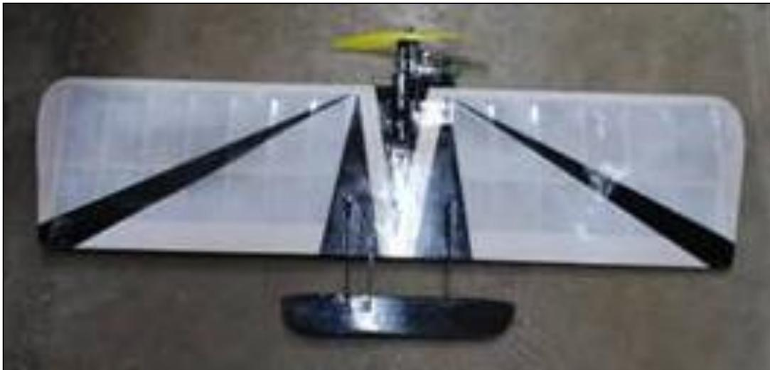
The clear material was given a mist coat of Rustoleum white primer before I ironed it on. No other adhesive was required. The material can be trimmed with dope, however this model is trimmed with black Econokote. If you check out the sources below, you will see that you can have a lifetime supply of this material for less than \$50.00.
