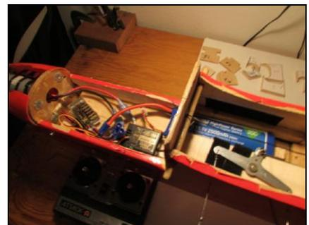
Upgraded to Solid State ESC and LiPol battery pack. that it cut the weight to 4 1/2 pounds. It flew, but still short of power. Brushless motor next.
