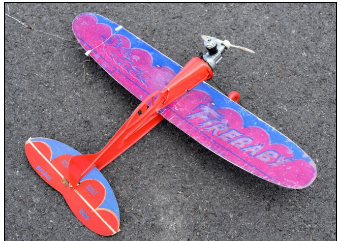
Gene Pape put together this vintage Jim Walker Firebaby from a box of parts he found on eBay. The wing is a new one Gene built, with graphics printed on an inkjet printer and applied to the wing. Gene made five flights on the Firebaby with the vintage Babe Bee engine. Flying Lines photo.
