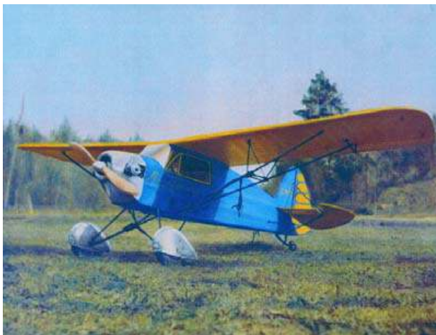
Miss Shirley, the first Control Line plane. It was designed and built by Oba in 1936 and 1937 for his Control Line invention.
