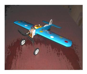
11.3 oz. RTF weight with 3 cell 1000 mah LiPol battery pack. The extra 3+ oz of weight should help with line tension, but most likely will hurt performance.
