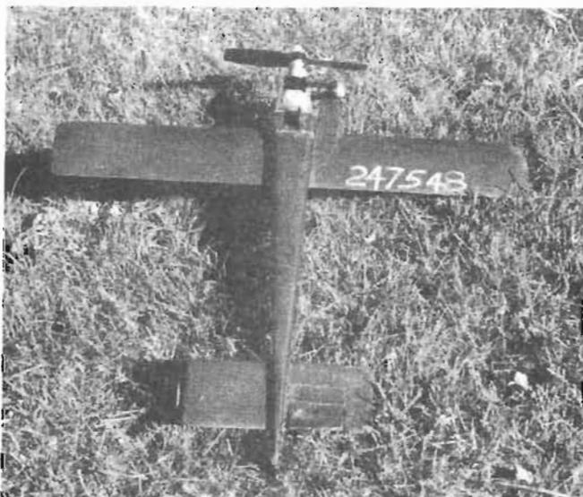
This small plane is the Mouse Racer that Joe and Paul Rice have used for a number of years, and has been a NW record holder a number of times. The design is original, and with a 28 square inch wing is a lot smaller than the ever-present Streakers that we see in the Mouse circles. The engine is a "KK" unit that began life at the '89 Nats, and uses a homebrew 57% nitro blend. While not currently a record-holder, this rugged plane will probably be a contender for some time to come.
