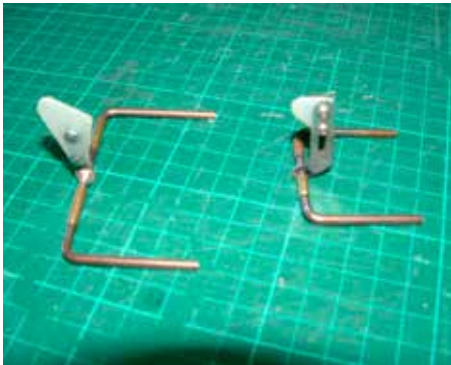
Nylon horn brackets are used to reduce friction and wear on the pivot joint. Brackets are cut from 2mm nylon sheet. Horns are cut from 1.2mm steel plate and silver brazed onto the 3.2mm mild steel wire.
