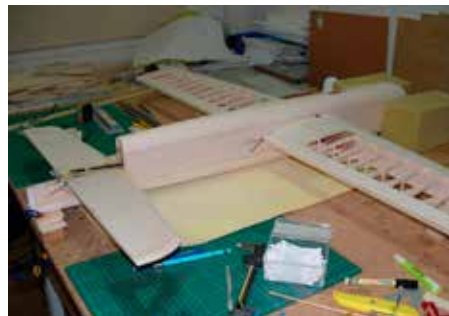
The top & bottom moulded shells have been glued onto the fuselage. The tailplane mounting plate is being glued in place after checking the tail alignment.
