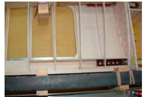
The rear wing joiner is glued in position between the trailing edge doubler and the vertical grain shear webbing.
