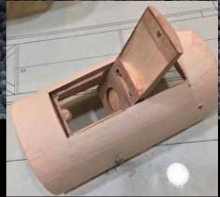
There are five hatches on this airplane: two elevator access hatches, an accelerometer access hatch, an arming plug and activation switch access hatch, and, of course, the battery hatch.
