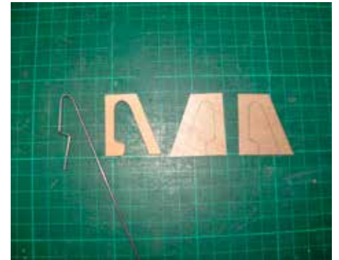
The removable tail wheel bracket pieces prior to epoxy gluing together. The inner piece is 1.6mm ply and the 2 outer pieces are 0.8mm ply.
