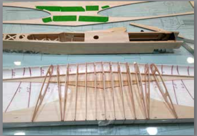
Note bottom bellcrank mount and geodetic structure in fuselage.
