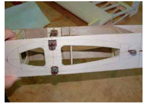
The take apart system for the wings uses my own design phenolic (Bakelite) joiners. The phenolic sheet is easy to cut on a band saw and the bolt holes don't require any bushings.
