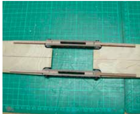
The phenolic wing joiners being test fitted to the main wing spars. The M4 connection bolts are loaded in double shear to ensure maximum strength and durability. The spars are made from 2.5mm balsa with partial span 0.4mm ply doublers each side.
