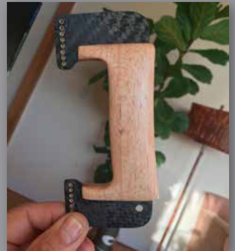
Cox/Resinger hardpoint handle modified with a Fancher style balsa grip.
