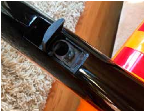
Hinged arming plug under swiveling magnetic hatch.
