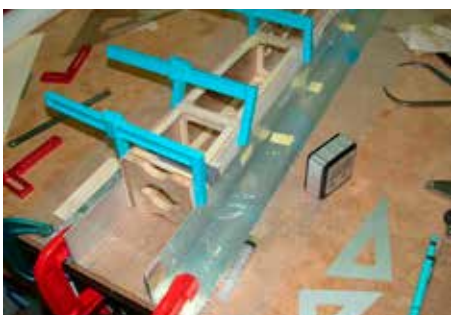
The plywood nose formers and the balsa/ply composite motor mount former being epoxy glued into position.
