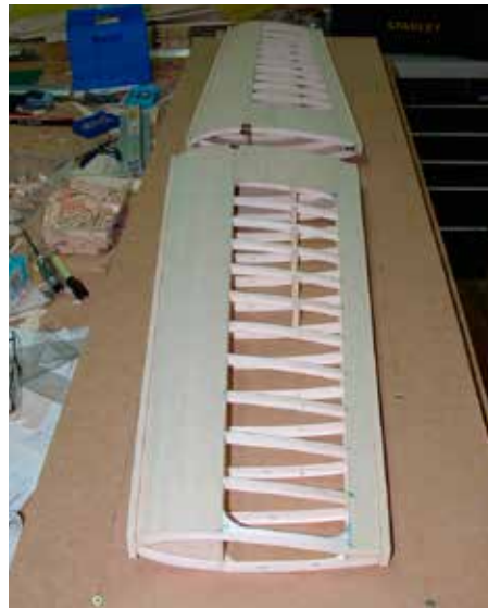
Wing panels are nearly complete. Leading and trailing edges need to be sanded to shape and then wing tips added.
