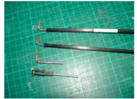
Pushrod ends are made from 2.4mm mild steel and glued into the carbon fibre tubes with JB Weld. The adjustable DuBro 4-40 nylon clevis has a removeable 1.6mm pin for connecting to the tail horn.
