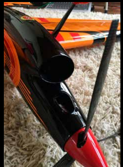
Cooling vent for motor and airscoop wick directs air over the ESC.
