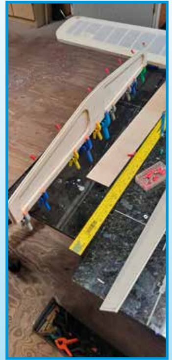
Stabilizer, Vertical Lamination. This was used to prevent distortion after curing. I have had problems with the flat surface and heavy weight method.
