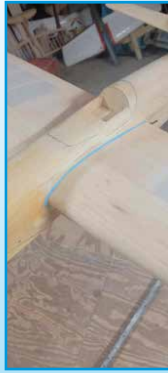
SuperFil is used to make fillet for wing to fuselage joint.
