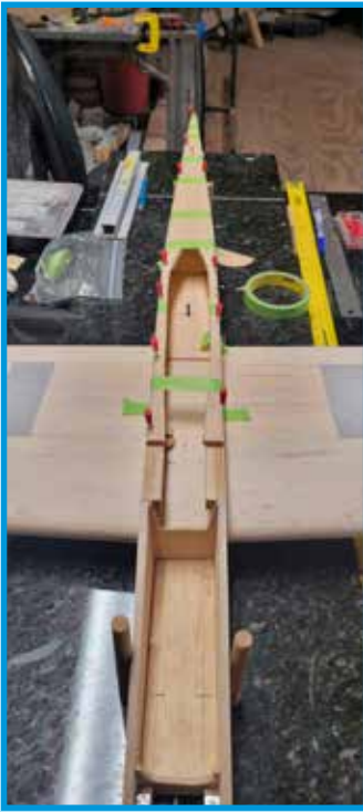
Balsa bottom block being glued on, after pipe floor installation.
