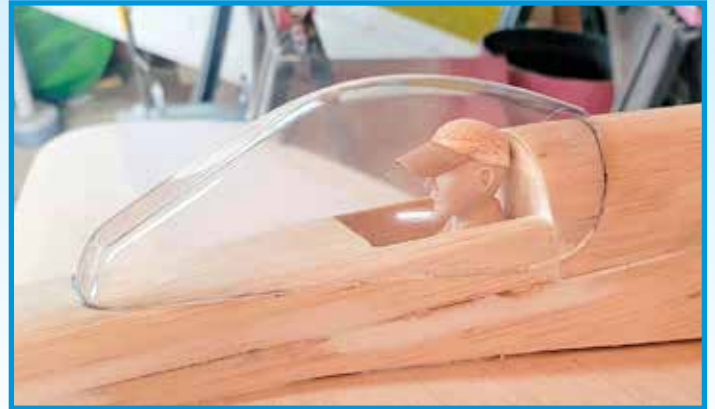
Test fit of Pilot and plastic canopy before painting.
