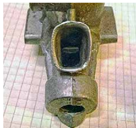
Inspired by American engines like Fox, the venturi intake was made big and rectangular. But also to test the principle to have the venturi look the same as the cut-out inlet in the crankshaft.
