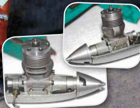
Glenn Lee USA and his side exhaust schnuerle K&B Wart engine.
