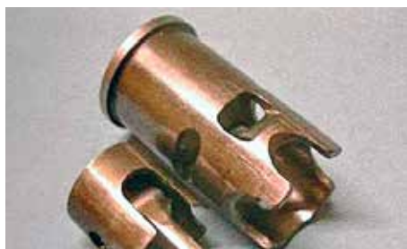
Several variants of porting with cut-aways in both the liner and the piston was tested.
