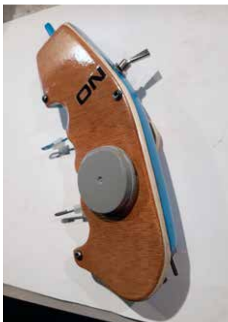
Example 1: Radio integrated in the handle. A simple and easy to build electronic circuit which controls the 2.4 GHz transmitter in On/Off mode, with the switch mounted on the handle, 100% controllable by the pilot.
