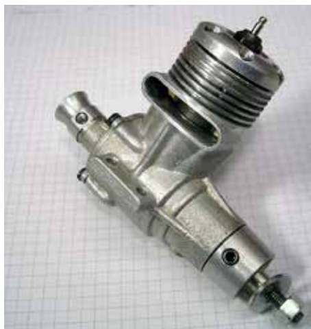
The rear intake side exhaust prototype with the venturi straight out from the back cover.
