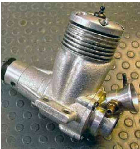
Another prototype with a rotating drum instead of a rotating disc as can be seen on the engine to the left.
