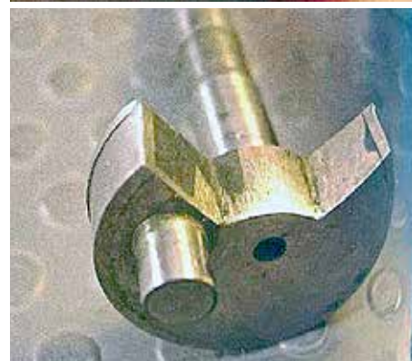
Photos showing the principle for the front intake disc system which gives balancing problems and also left the engine without a rear ball bearing.
