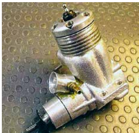
The front intake engine with a front rotary disc as you can see from the position of the venturi.
