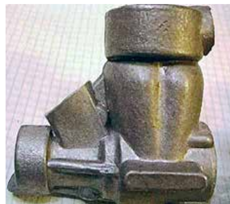
Prototype casting of an engine with a big square intake, later abandoned. Also note the tests with bilateral ports in the crankcase although it has unilateral porting.
