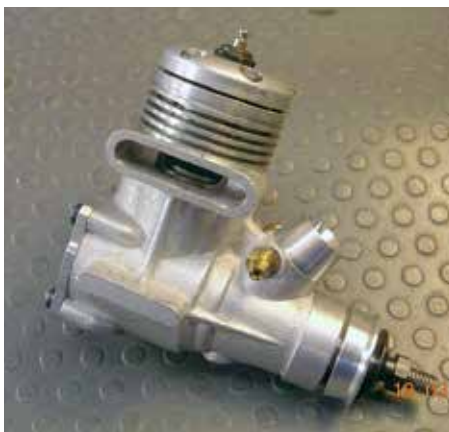
Back to a conventional crankshaft with intake inside the shaft. Note the reinforced front part of the crankcase.
