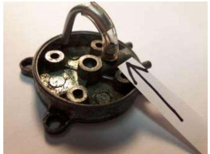
**Incorrect fuel attach tubing allows for leakage at the backplate nipple as well as where it attaches to the aluminum pick up tube.**
