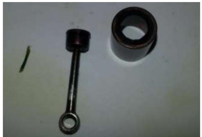
**Above: This is what happens when one neglects the resetting of the ball-socket joint of a Cox .049. Ingested grass is bad too.**
