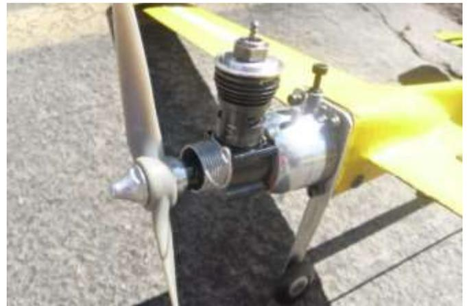
**The business end of The Gibeault "Streaker V" entry. \*Note the Doug Galbraith head fitted with a Nelson glow plug that costs half the price of a Cox glow head. This Cox Venom uses a stock Cox 5-40 stud screw & Cox spinner to avoid crankshaft shearing & sheet L.G for improved drag reduction.**
