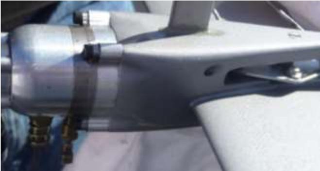
**Note venturi air hole in fuselage just ahead of the bellcrank slot.**
