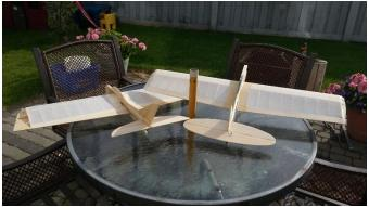
Both Flite Streak & Ringmaster are drying outside after the Polyspan has been applied.
