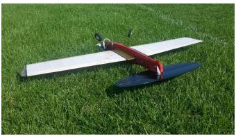
**Ringmaster: Full power on crash with no wing damage** (will need LG & prop work thought)
