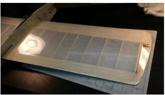
Finished! The SLC covering goes on very easily over the bare Polyspan.
