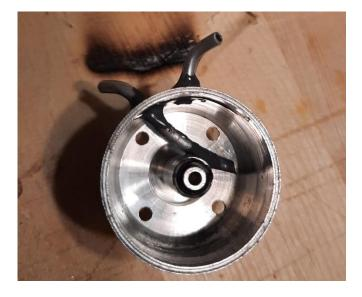
Finally, I put together another Cox 049 for my mouse. That last motor I had worked well (for me at least) it revved up to 19.5k and ran a consistent needle the entire tank but was lost when the motor was stopped incorrectly after starting backwards. I made a uniflow tank like the one on my last motor and hopefully it will run as good. Many thanks to Bill Bischoff and Dave Hull for their hardware and advice. Happy trails and Merry Christmas.
