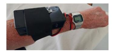
The LEDs are on the side of the box. If you look at where the battery ends up when it is strapped to my arm, the LEDs are always visible out of the corner of your eye when servicing the model. Coupled with the extreme brightness of the LEDs, confirmation of the glow plug is always there without any extra motion for the pit man.
