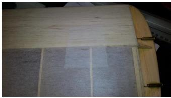
"Hangar Rash" shop punctures are a snap to patch at this stage.
