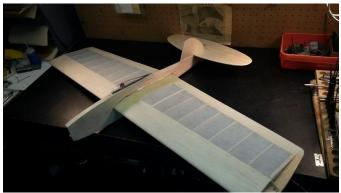
Here the Polyspan has been heat shrunk & edges trimmed.
