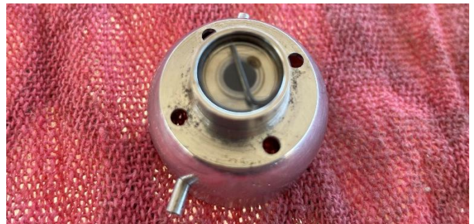
Doug's Mouse 1 fuel tank showing the rock trapped underneath the reed.
