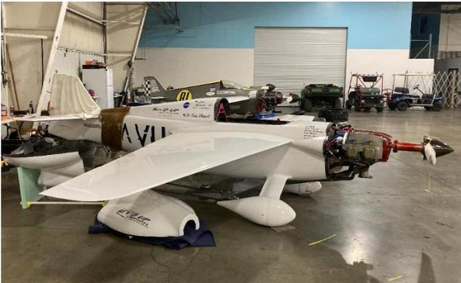
“Déjà vu” with cowling removed showing prop extension and Exhaust routing.
