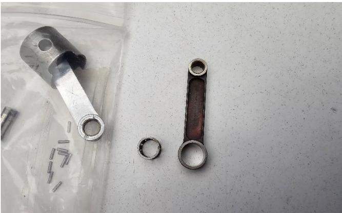
**One version of this engine used a needle bearing connecting rod. I understand, the bearing roller cage is one of the more difficult/delicate parts to make. I don't know if the roller bearing rod was worth all the extra effort compared to the regular type of rod.**
