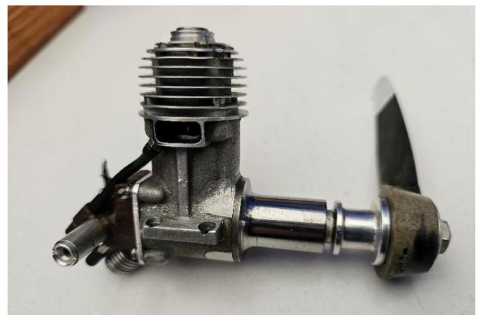
I had the very good fortune recently of being able to have a look at this FMV T/R engine belonging to Hans Visser. This particular example was essentially a de-bored 2.5cc engine if I understand it right. Of course the thicker cylinder liner made for a very nice engine to set and run. Unlike the 2.5 engine, this example employed a single blade prop that worked very well in this class.
