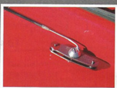
This beautiful bellcrank assembly by Darrel Albert is used on both ships.
