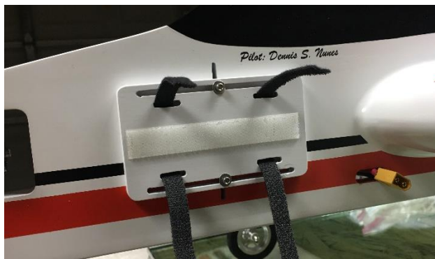
Figure 22 - Battery Holder Ready for a Battery
