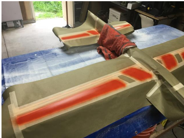
Figure 14 - Applying the Madrid Red Trim Color (Circulas 61)
