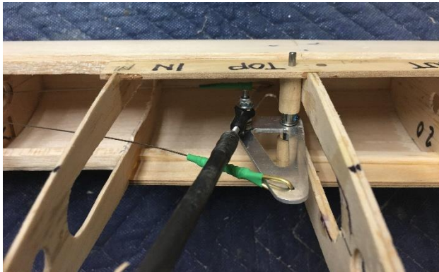
Figure 15 - Aluminum Bellcrank Installed
