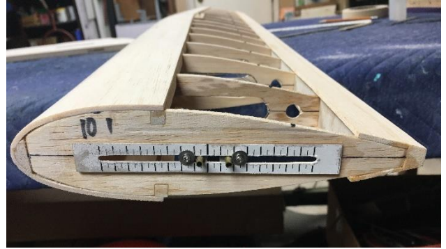
Figure 22 – Installed Adjustable Leadout Guide
