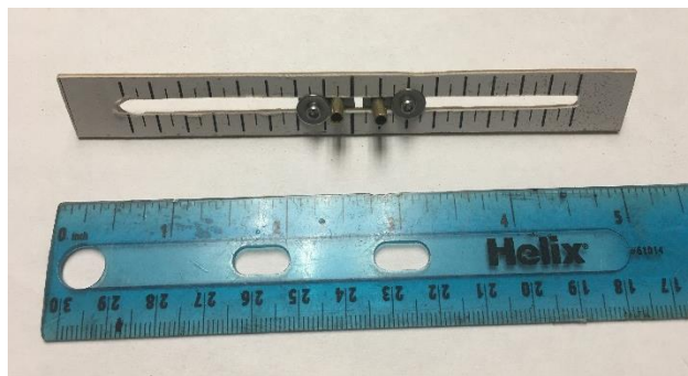
Figure 21 - Finished Leadout Guide
