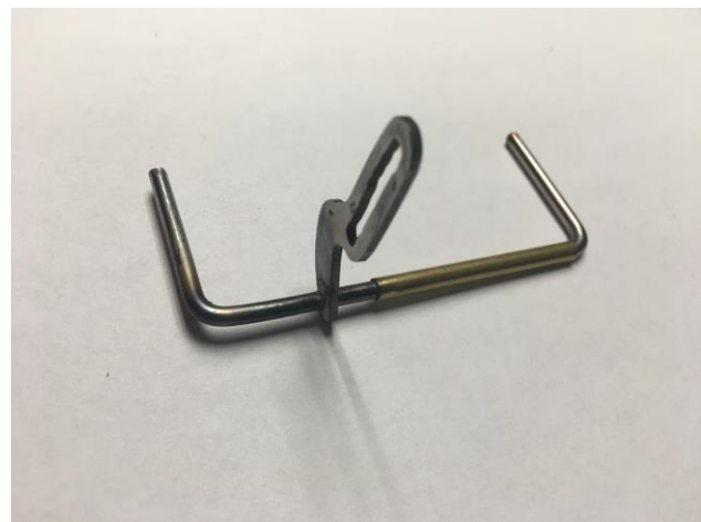
Figure 16 - Finished Elevator Control Horn
