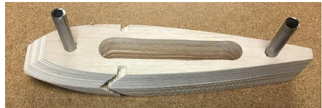
Figure 9 – Cut Out the Center Portion of the Ribs
