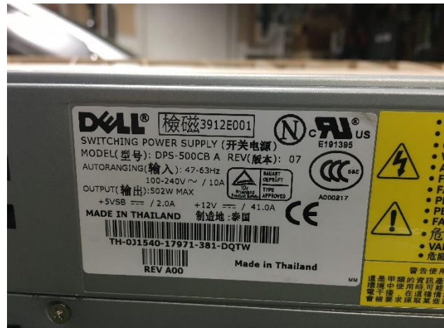
Figure 2 – Power Supply Type
