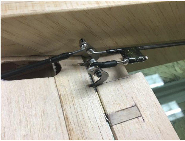
Figure 32 - Fitting of the Flap Horn (Note the notch in the flap to clear the WFAD)
