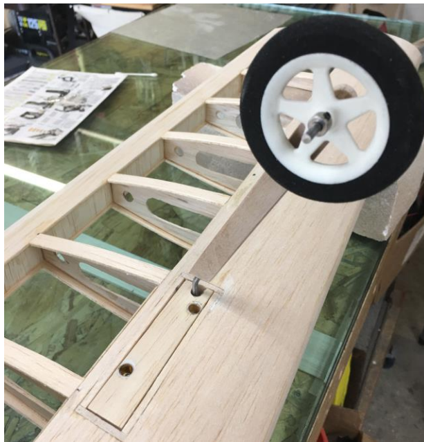
Figure 6 - Installed Landing Gear with Fairing and Cover
