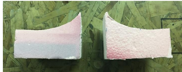
Figure 13 - 2" Thick Styrofoam® Supports
