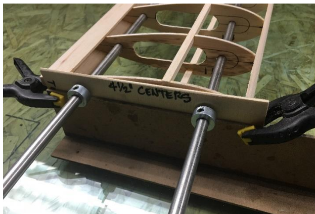
Figure 5 - Wing Jig End Caps Locked Down
