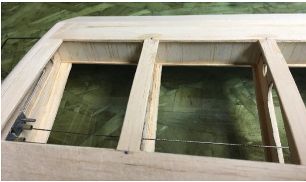
Figure 24 - Shear Webbing at Trailing Edge
