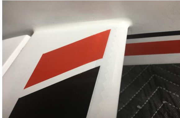
Figure 6 – Installed Trip Strip (maybe difficult to see)
