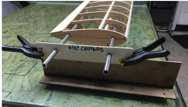
Figure 4 - Wing Jig End Cap Clamped to End Support
