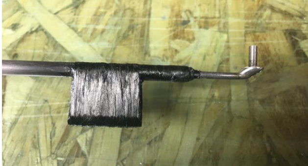
Figure 22 - Wrapping with Carbon Fiber Tow and Soaked with Thin CA
