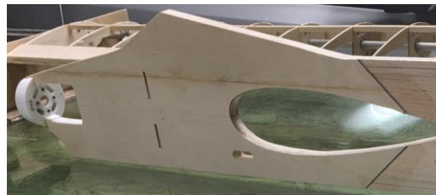
Figure 10 – Fuselage with Plywood Doublers
