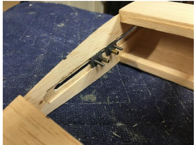
Figure 23 - Backside of Installed Leadout Guide
