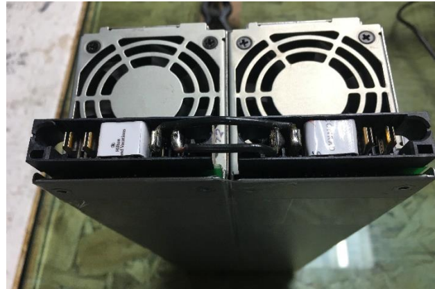
Figure 8 – Plastic Isolators over Pins
