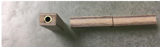
Figure 29 - Control Horn Drivers Cut to Length
