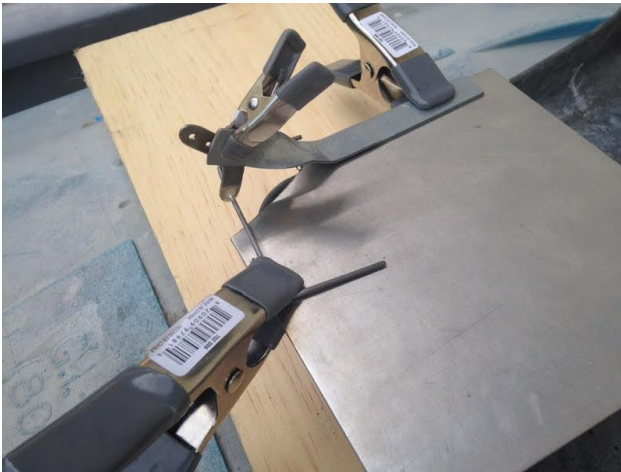
Figure 14 – Holding Jig (Photo from VCB Weekly NAG 8-14-17)
