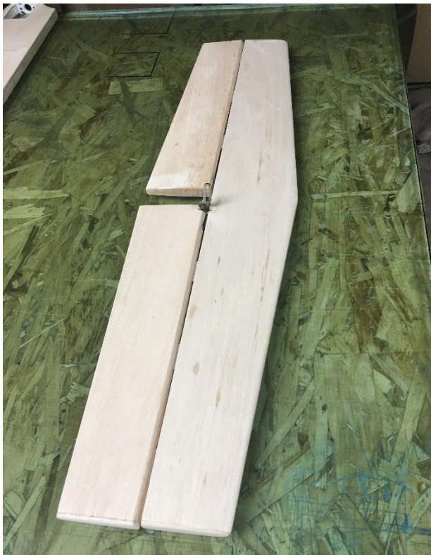
Figure 22 – Finished Stabilizer and Elevators
