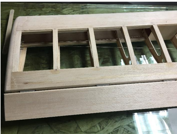
Figure 26 - No Shear Webbing at Last 4 Bays of Inboard Wing
