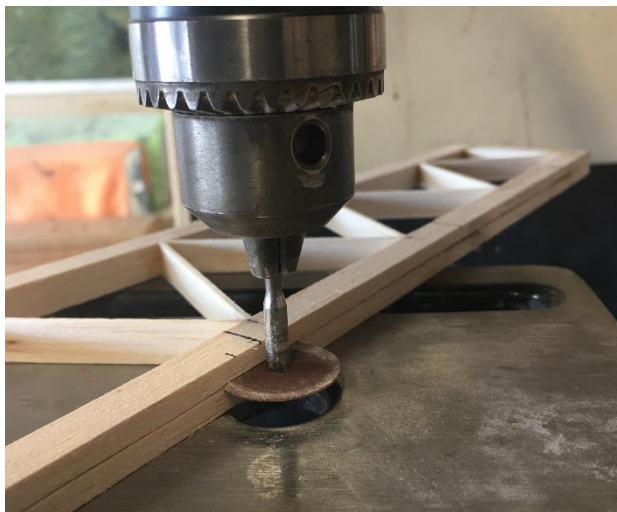
Figure 19 – Cutting Hinge Slots with a Drill Press
