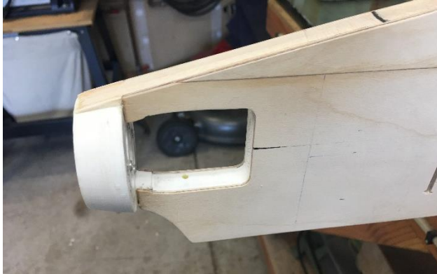
Figure 11 – Finished Installation of 3D Motor Mount
