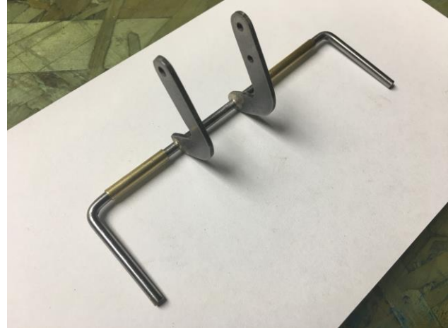
Figure 15 - The Finished WAFD Flap Control Horn (Before Being Split)
