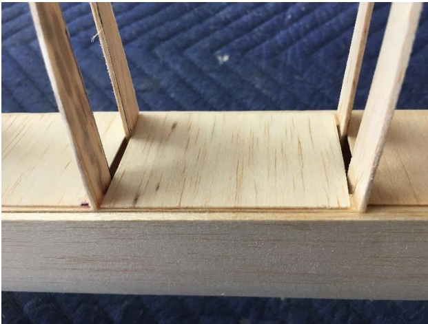
Figure 25 - Shear Webbing Between the Spars
