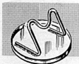
Neat soldering iron rest from coat hanger wire and tin lid. Stan Bidowski, Winnipeg, Manitoba.
