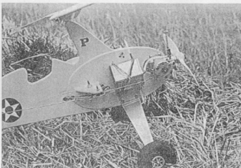
Close-up of the front end showing engine and tank installation—note throttle control.
