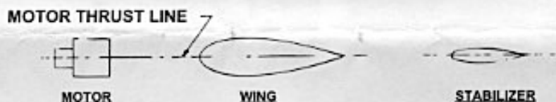
EXAMPLE #1 • MOTOR, WING AND STABILIZER ALL ALIGNED ALONG SAME THRUST REFERENCE LINE
