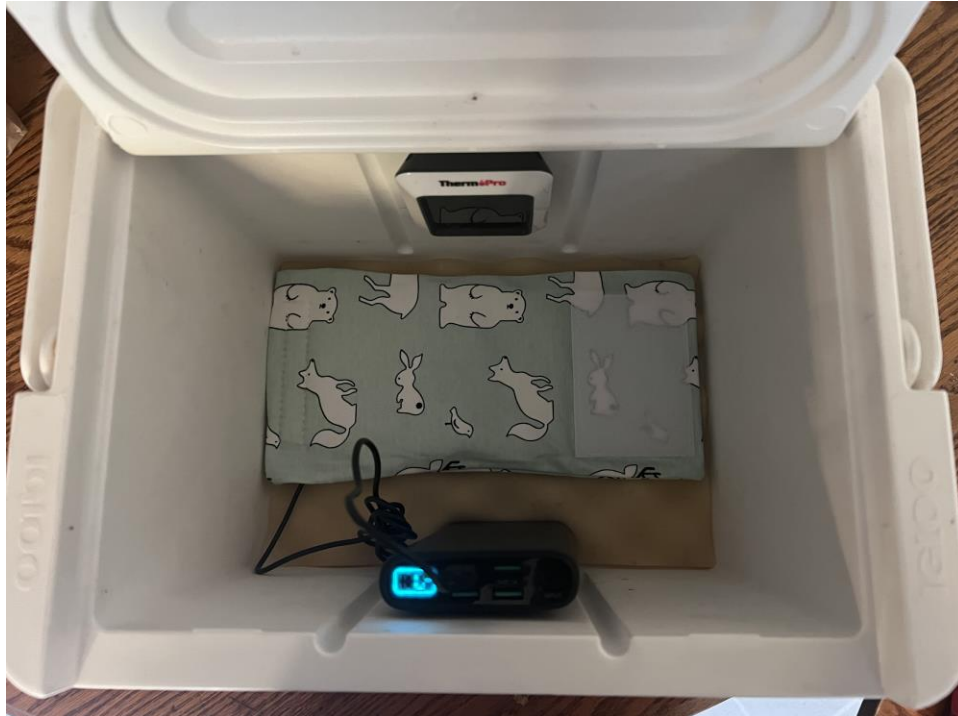
An Inside View of my Battery Warmer, without the Batteries
